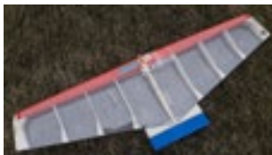
Models F2D with integral elevator and carbon trailing edge + full kevlar wrapping
