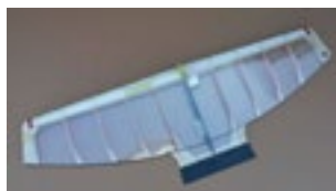
Models F2E "Ras-tenis" DIESEL 2.5cc with metal tank spars fiberglass, foam EPP, carbon elevator
