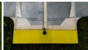
Models F2D with integral elevator and carbon trailing edge + full kevlar wrapping
