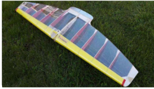
Models F2D Andrej Beljaev with carbon trailing edge and full kevlar wrapping
