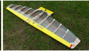
Models F2D Andrej Beljaev with carbon trailing edge and full kevlar wrapping
