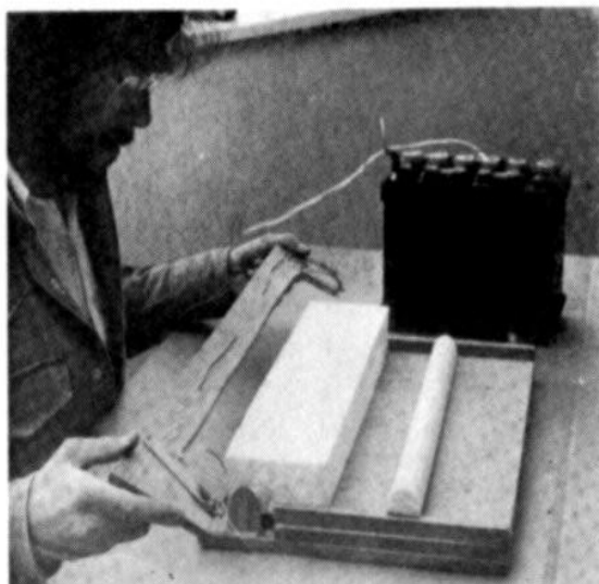
Forming the leading edges from expanded polystyrene is very quick and easy, the only tools necessary being those that you can make yourself. A car battery is used to supply the heat for the hot-wire cutter - how to do it will be described in the May issue.
