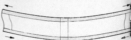
Figure 5 – showing how flanges distort flexible tip webs.
