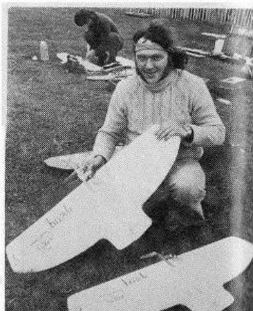
Dave Willis with his Rossi powered Boomerang models, glass cloth centre covering made them really tough, used vac-formed pacifier pods soon to be commercially available.
